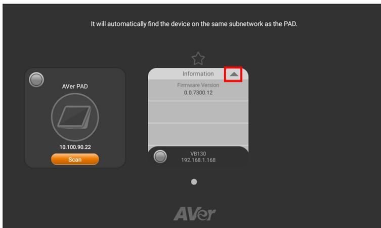
4. Tap **Set IP** to set the camera's IP. The Web page access password of camera needs to be entered to continue. (If you have not set up web page access password, the default is aver4321.)
