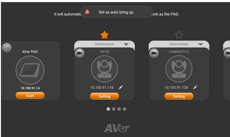
8. Tap **Setting** to enter the setting page of the camera. If it is the first time accessing the camera, you will be required to input camera's default web page password (aver 4321) and set a new account and password.
